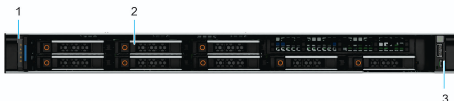
Figure 2. Front view of 8 x 2.5-inch drive system
