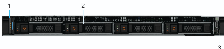
Figure 1. Front view of 4 x 3.5-inch drive system
